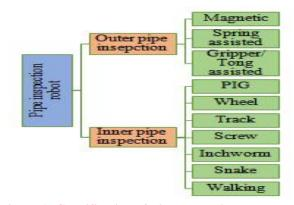
Figure 1: Classification of Pipe Inspection Robot.
